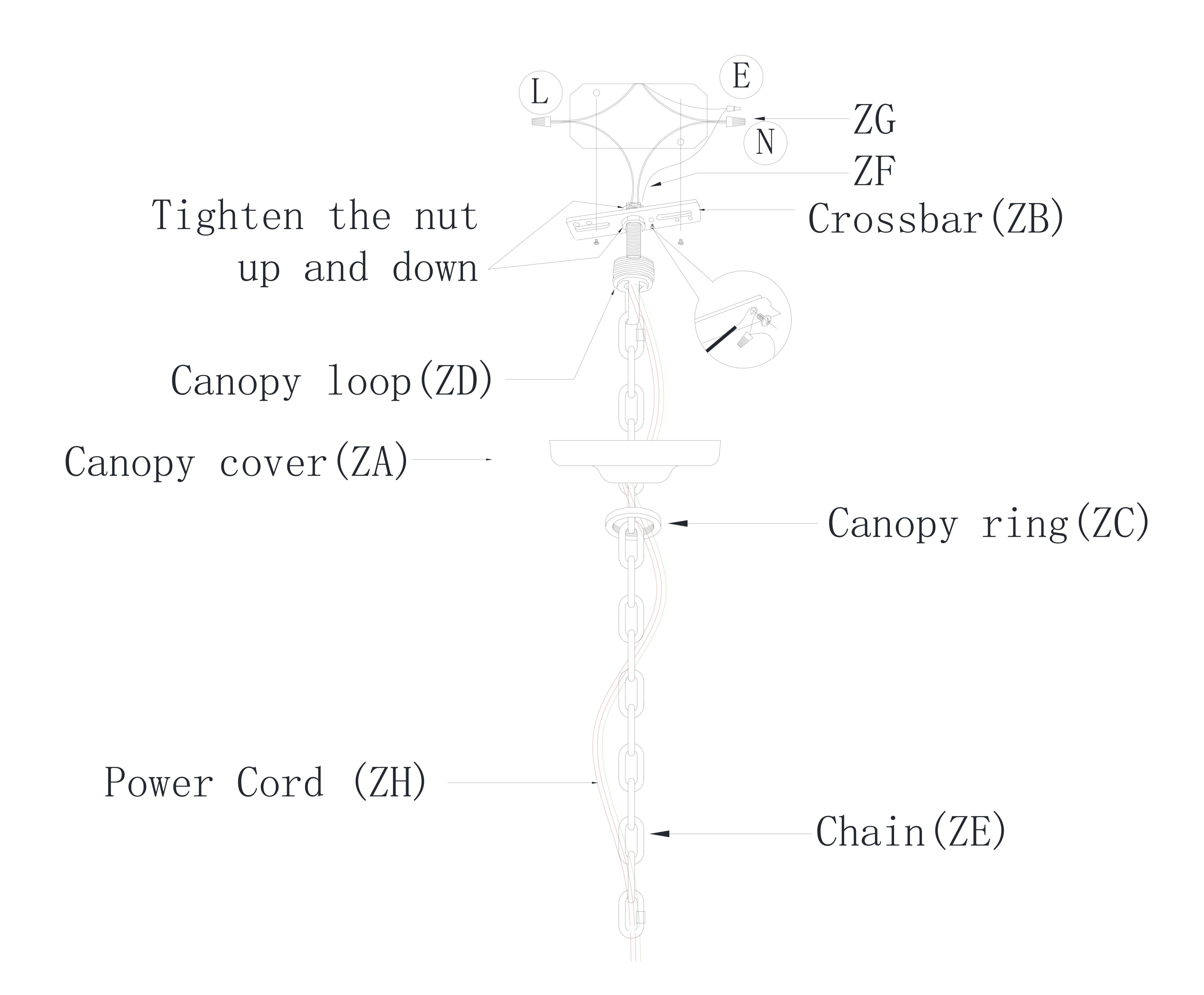
IMPORTANT: Test sockets with bulb before dressing the fixture.
